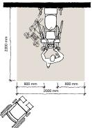
Grey area shows the minimum working area required for the staff to be able to use the mechanical aids in an ergonomic way from one side.
